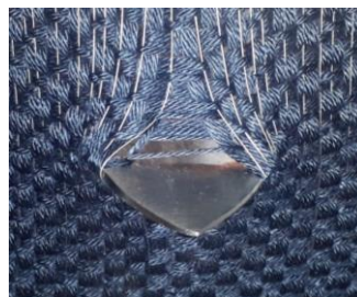
Fig. 6: Deformation of fabric structure during knife penetration into the fabric
